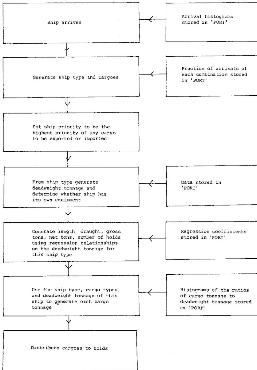
Figure 2: Procedure for Generation of Ship's Characteristics
