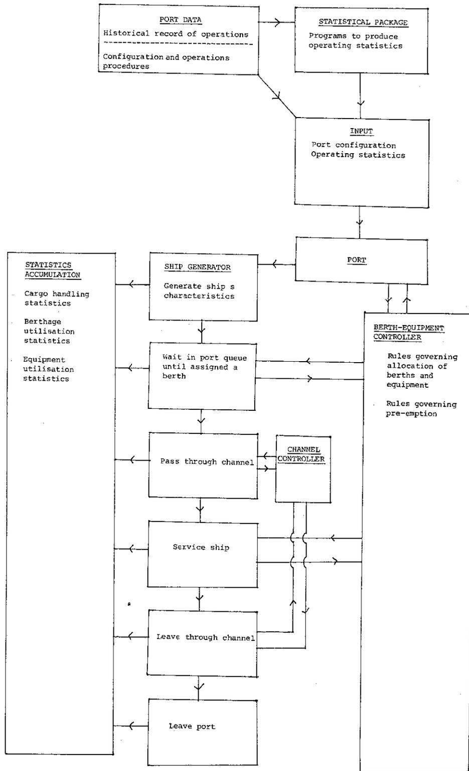
Figure 1: Structure of the Port Simulation Model
