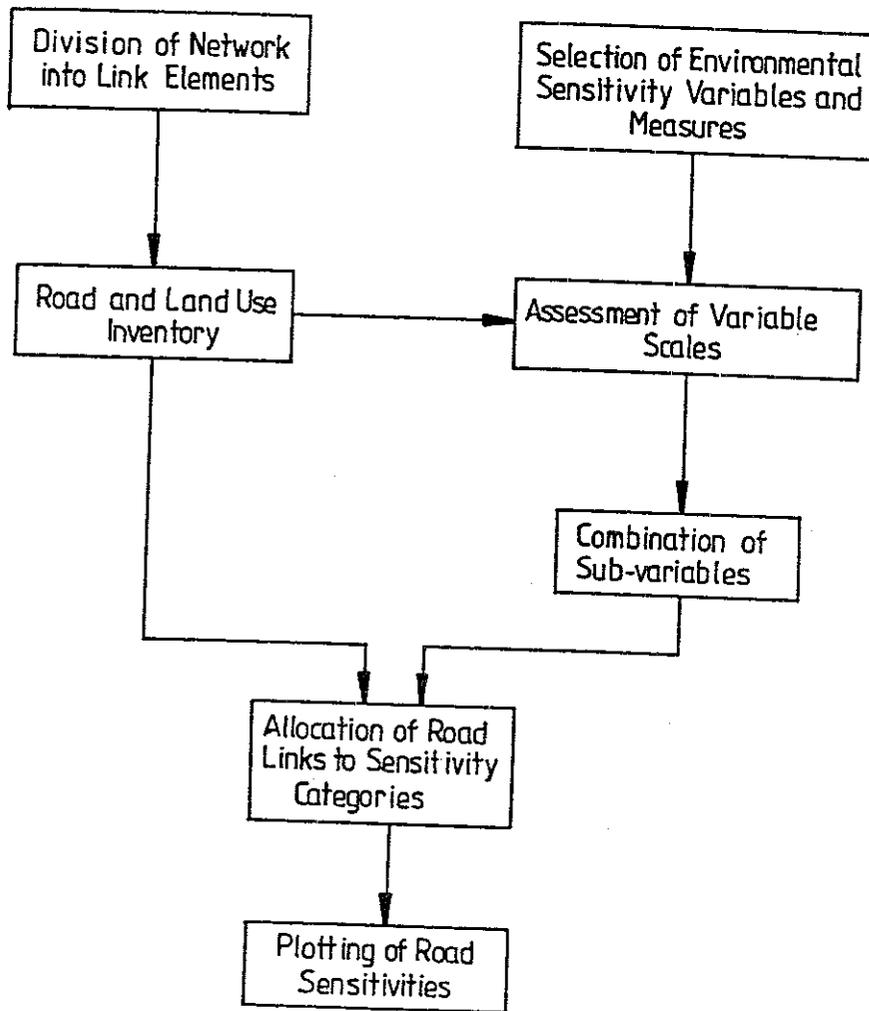
Figure 2: Environmental Sensitivity Methodology
