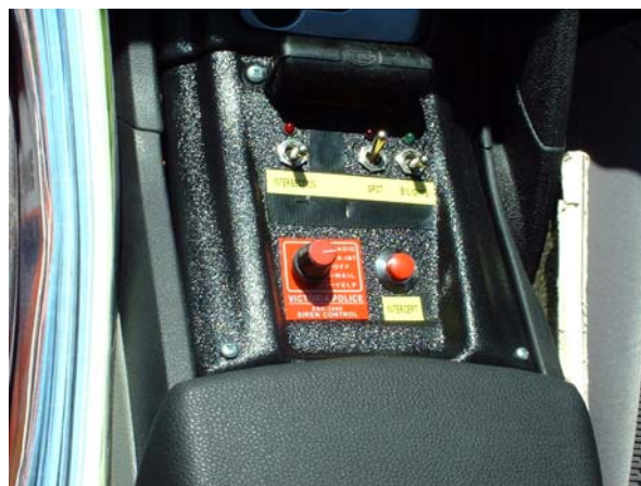
Figure 4 – Victoria Police in-vehicle EVP switch
