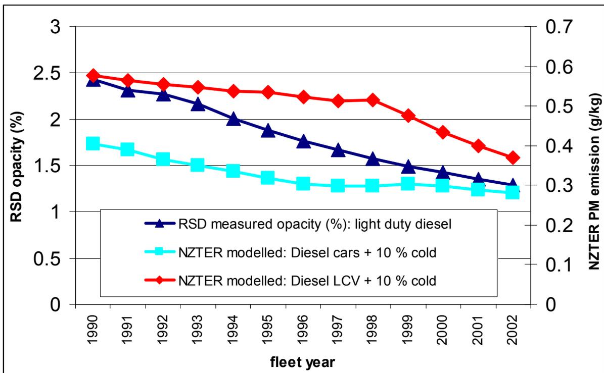
**Figure 7 Comparison of trends in measured opacity and modelled particulate emission rates for light duty diesel vehicles**
