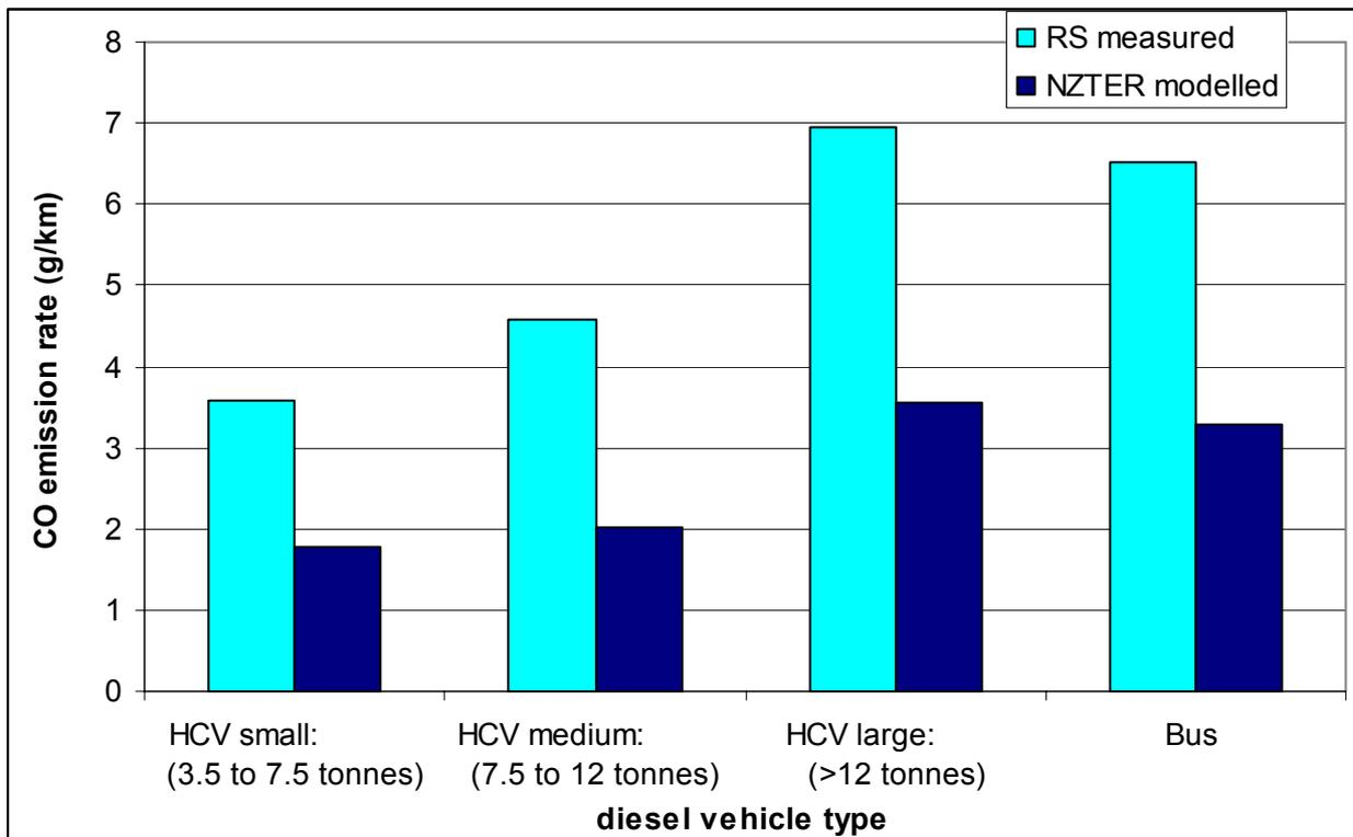
**Figure 6 Comparison of NZTER modelled and RSD measured CO emissions for diesel HCV and buses**
