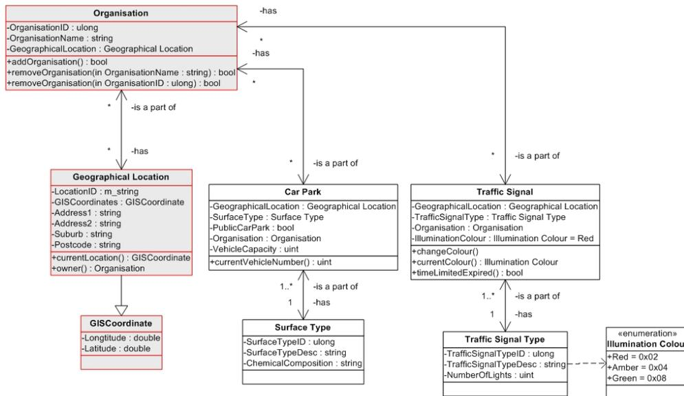
**Figure 4** A sample class-object diagram for the car park/traffic signal objects
