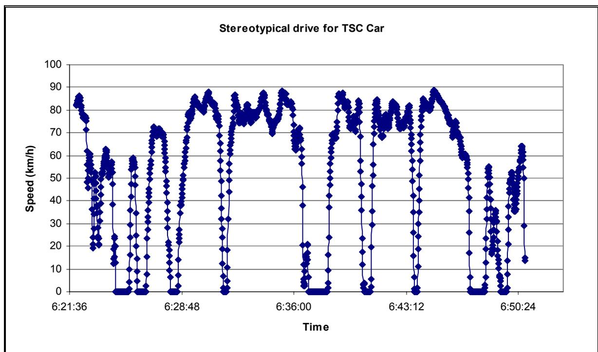
**Figure 9 Stereotypical drive for TSC car**
