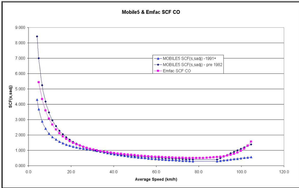
Figure 1 Mobile 5 Speed Correction Factors for CO
