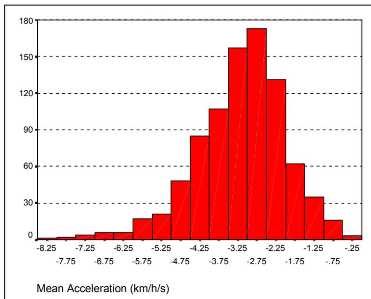
**Figure 8. Number of Deceleration-to-Idle phases categorised by acceleration.**
