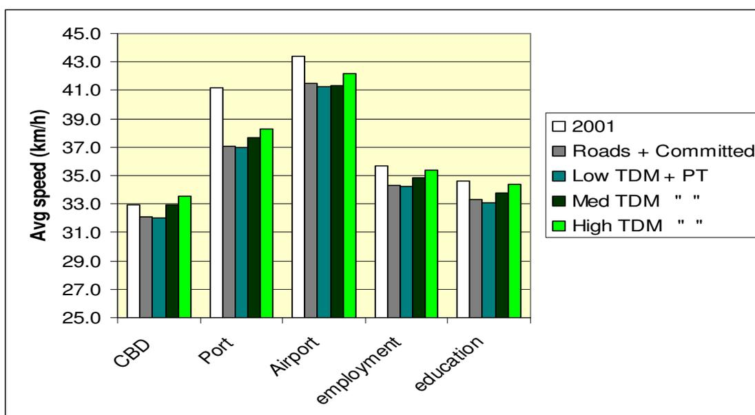
**Figure 2: Congestion impacts - Average vehicle travel speeds to/between key economic centres<sup>9</sup> for TDM options in 2016 compared with 2001.**
