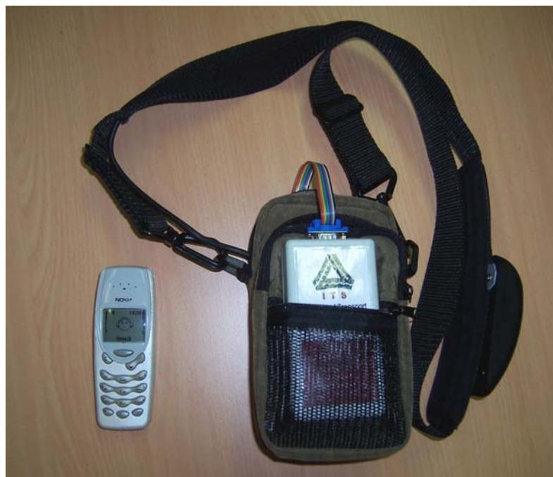
**Figure 2: Early Wearable GPS Device Shown by a Mobile Telephone**
