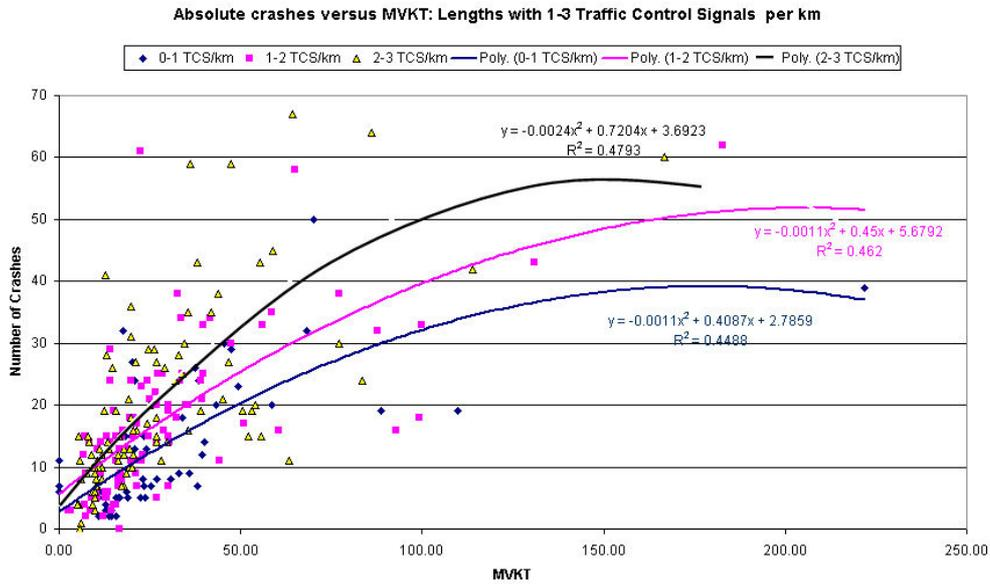
**Figure 4 Absolute crashes versus MVKT for segments with 0-3 traffic control signals per kilometre**
