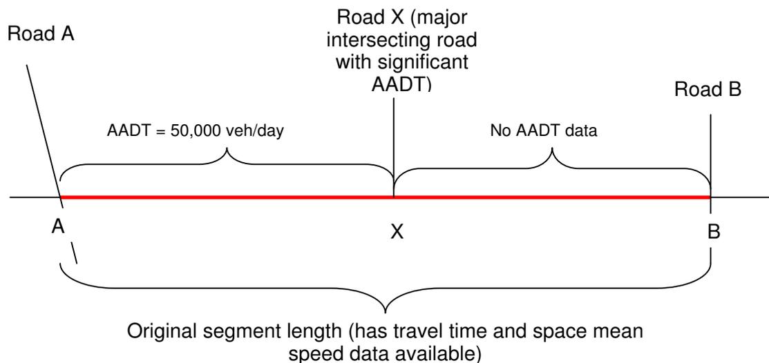
In this example, travel time and space mean speed data available for the whole length A-B. However, traffic volume data is only available for A-X. Furthermore Road X is a major intersecting road which carries a significant traffic volume (AADT). Therefore, the revised segment length would be A-X and the travel time information would be derived by dividing the length A-X (km) by the space mean speed for A-B (km/h)
