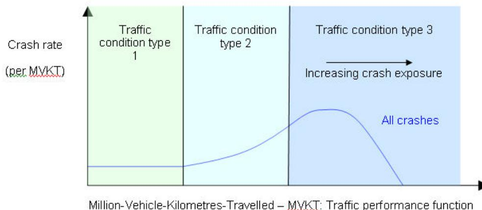
**Figure 2 The hypothesised relationship between crash rate (per MVKT) and MVKT (as a function of traffic flow condition).**
