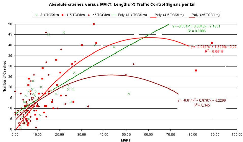
**Figure 5 Absolute crashes versus MVKT for segments with more than 3 traffic control signals per kilometre**
