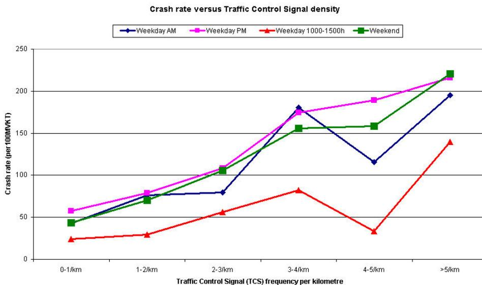
**Figure 9** Average crash rate versus Traffic Control System frequency.
