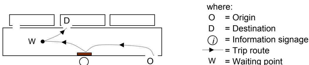
Figure 1 – Origin and Destination of trip segment at platform
