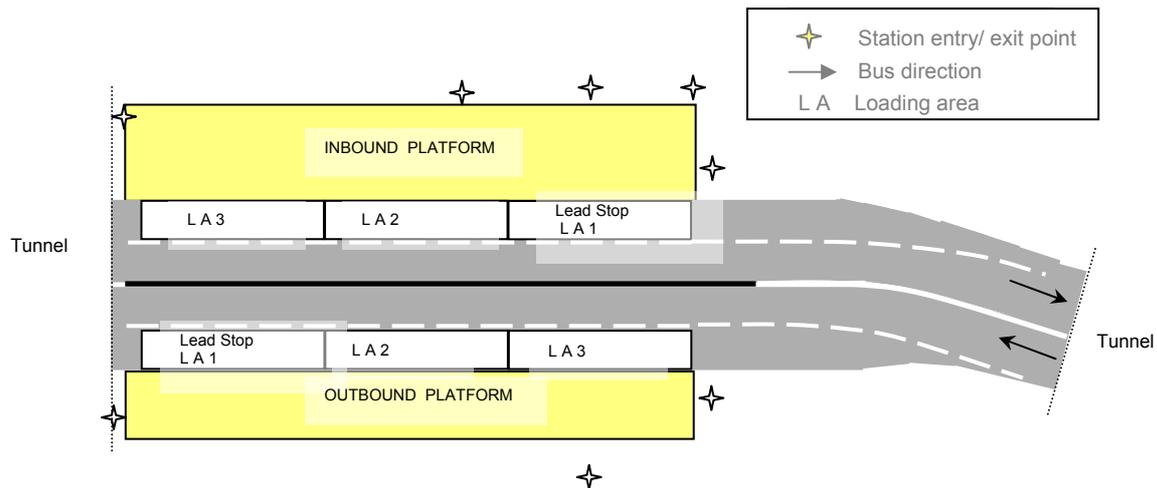
**Figure 3 – Configuration of Mater Hill busway station**
