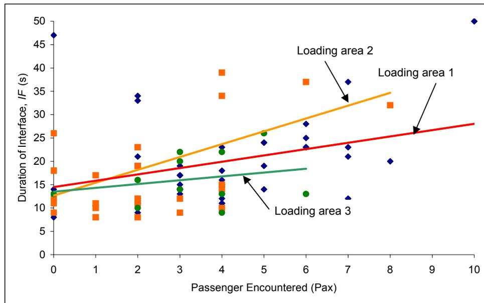
**Figure 8 – Effect of passengers encountered on platform on duration of interface**
