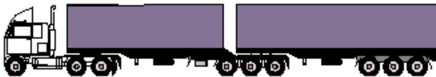
Figure 1: Super B-Double (non quad axle) configuration. A PBS Vehicle
