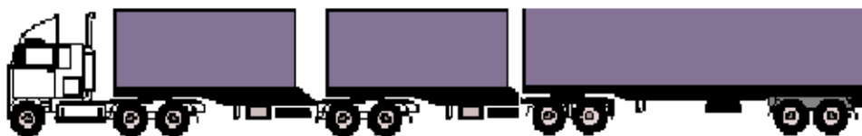
Figure 2: B-Triple Tandem configuration. A PBS Vehicle
