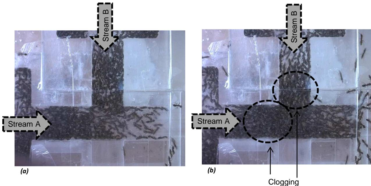
**Figure 4: Occurrence of clogging; (a) – Approximately 2 seconds after starting the experiment, (b) – Approximately 10 seconds after starting the experiment.**
