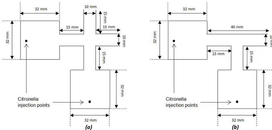
**Figure 1: Schematic diagram for the experiment setups; (a) – right angled crossing flows, (b) – right angled merging flows.**
