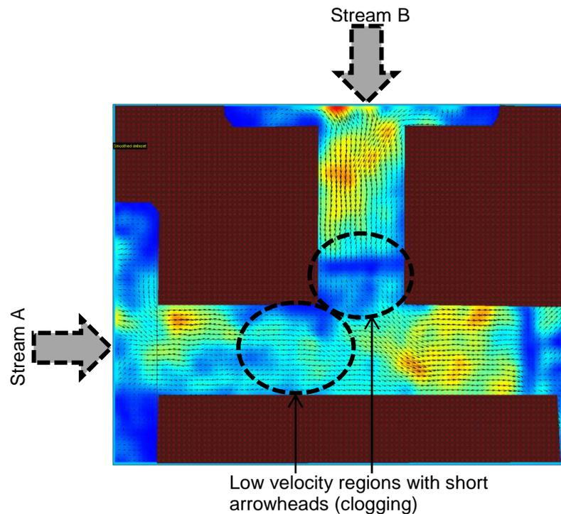
**Figure 5: 2D mapping of velocity vector fields for merging flows.**
