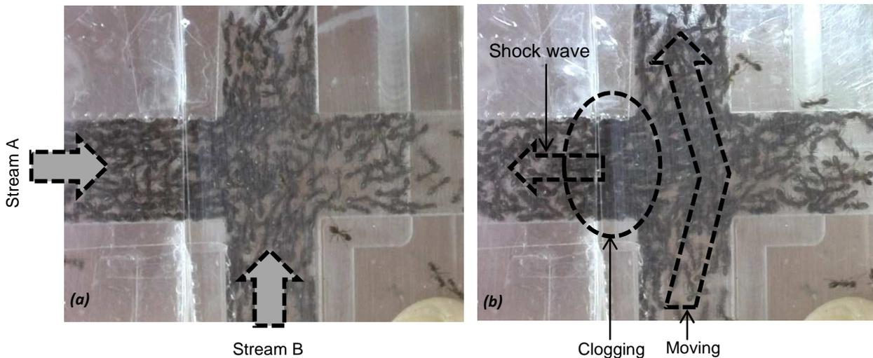
. Figure 2 Occurrence of clogging; (a) – Approximately 3 seconds after starting the experiment, (b) – Approximately 4-5 seconds after starting the experiment.
