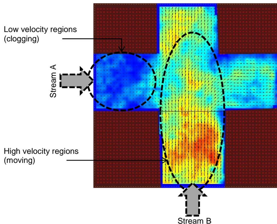
Figure 3: 2D mapping of velocity vector fields for intersecting flows.
