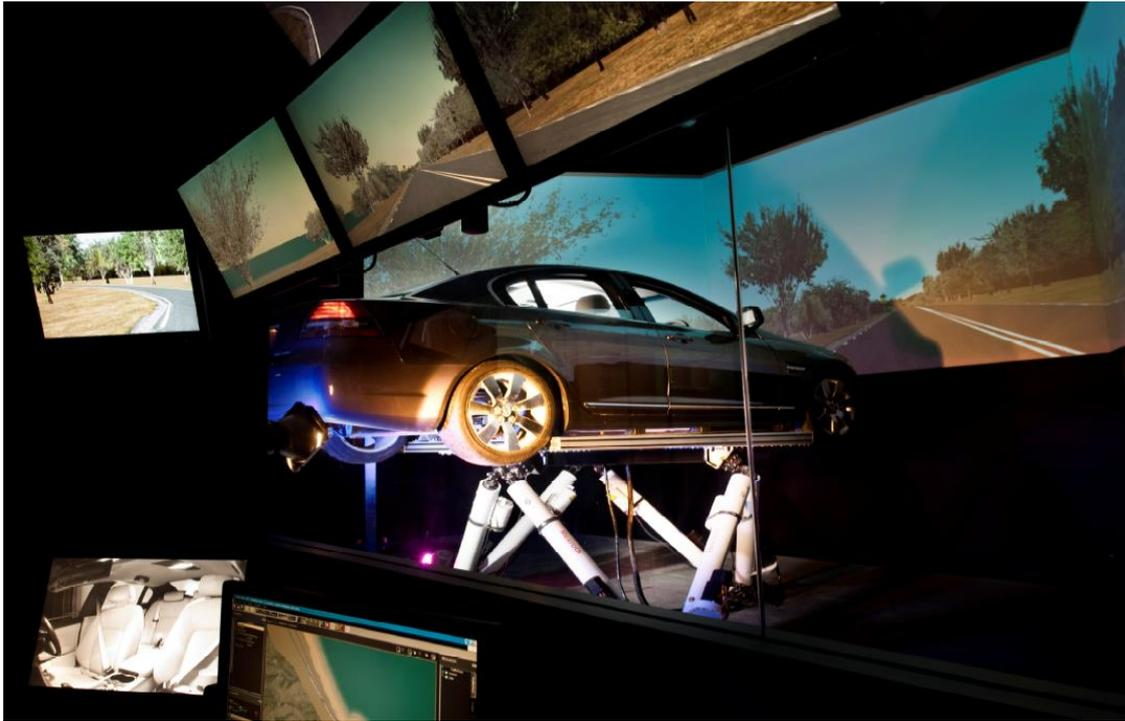
**Figure 1 Driving simulator at Carrs-Q**
