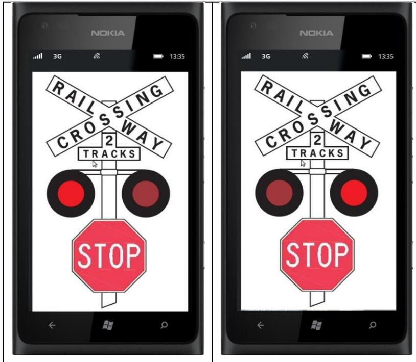
Figure 3 Capture of the in-vehicle visual ITS (train approaching and congestion)
